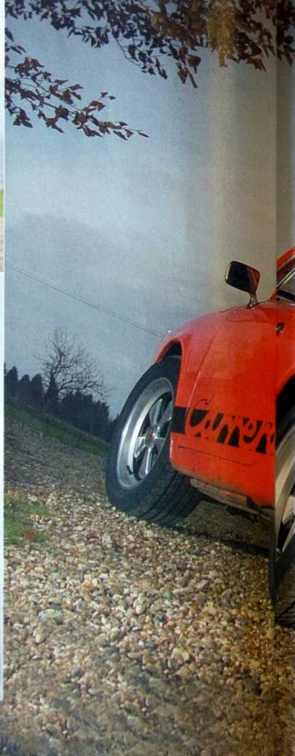
Above: Those Fuchs are the real deal and have been expertly re-anodised by Biaggio (see copy for contact). Bodyshell is originally that of a 1970 911T but with the correct RS spec steel rear arches. Exhaust is by American manufacturer Timmings
