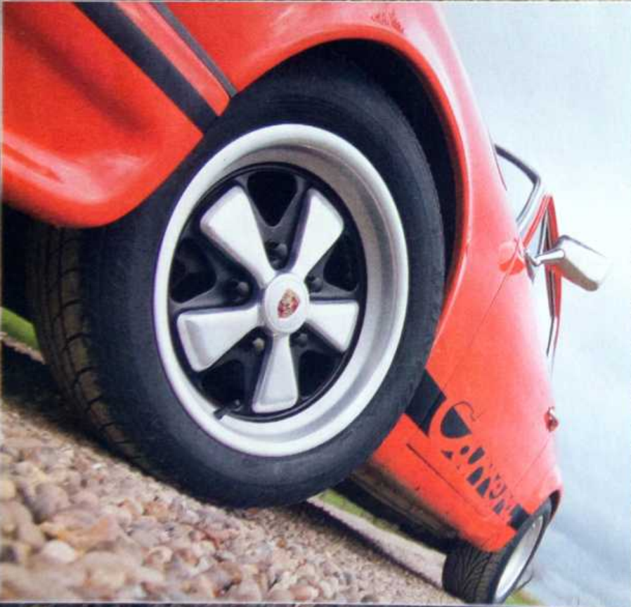
Above: Those Fuchs are the real deal and have been expertly re-anodised by Biaggio (see copy for contact). Bodyshell is originally that of a 1970 911T but with the correct RS spec steel rear arches. Exhaust is by American manufacturer Timmings
